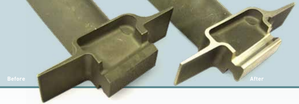
Fir tree before and after grinding
